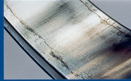
■ Phenomenon: Scuffing on Inner Ring Bore Surface ● Cause: Excessive Interference Fit with Shaft
