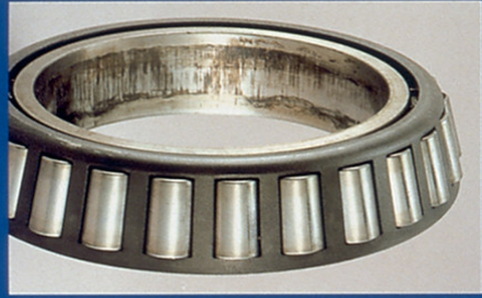
■ Phenomenon: Fretting Corrosion (Left)/Creep (Right) on Inner Ring Bore Surface ● Cause: Less Interference Fit with Shaft
