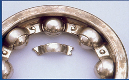
■ Phenomenon: Retainer Broken ● Cause: Abnormal Load due to Misalignment
