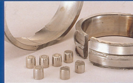
■ Phenomenon: Cracks and Chips on Inner and Outer Rings and Rollers (Left)/Seizure Caused by Chips on Ribs (Right) ● Cause: Excessive Axial Impact Load
