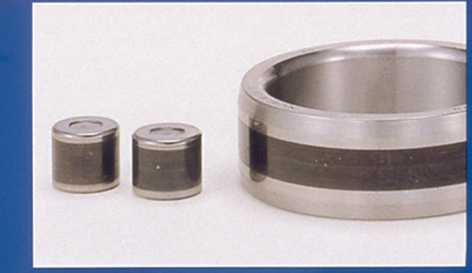
■ Phenomenon: Electric Pitting (Pit or Ridge-) and Staining ● Cause: Current Passed Through Inside of Bearing
