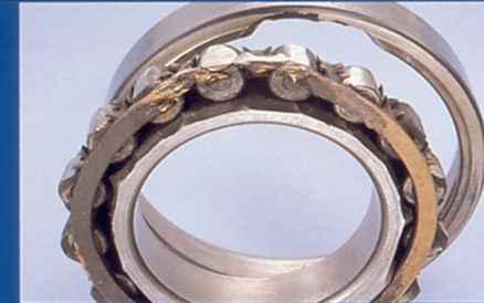
■ Phenomenon: Cracks and Chips on Inner and Outer Rings and Rollers (Left)/Seizure Caused by Chips on Ribs (Right) ● Cause: Excessive Axial Impact Load
