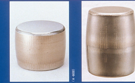
■ Phenomenon: Electric Pitting (Pit or Ridge-) and Staining ● Cause: Current Passed Through Inside of Bearing
