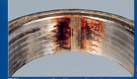
■ Phenomenon: Scuffing on Bore Surface ● Cause: Diagonal Assembly or Foreign Matter on Fitting Surface
