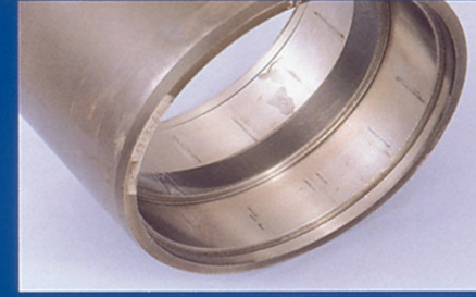
■ Phenomenon: Rust Generated on Raceway at Intervals on Roller Pitch ● Cause: Bearings Left Unused for Long Period under Moist Conditions
