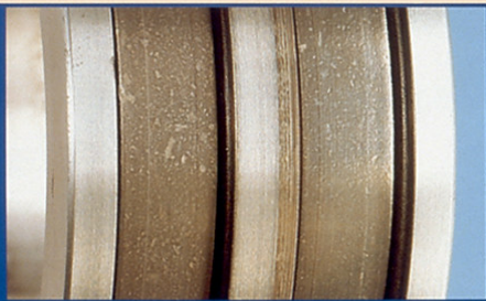
■ Phenomenon: Indentations on Raceway ● Cause: Contamination by Foreign Matter or Flakes from Other Bearing
