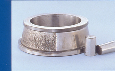
■ Phenomenon: Flaking Generated Around Half the Raceway ● Cause: Flaking Caused by Rust
