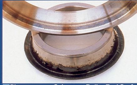
■ Phenomenon: Seizure at Roller End Surface and Inner Ring Rib ● Cause: Insufficient Bench End Play
