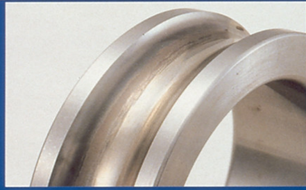
■ Phenomenon: Smearing on Raceway ● Cause: Improper Preload
