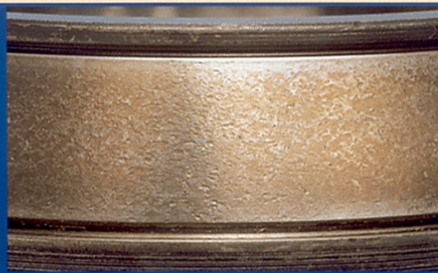
■ Phenomenon: Indentations on Raceway ● Cause: Contamination by Foreign Matter or Flakes from Other Bearing
