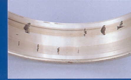
■ Phenomenon: Rust Generated on Raceway at Intervals on Roller Pitch ● Cause: Bearings Left Unused for Long Period under Moist Conditions
