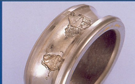
■ Phenomenon: Flaking at Intervals on Ball Pitch ● Cause: Indentations Caused by Impact Load Develop into Flaking
