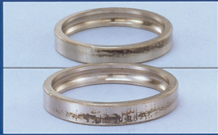
■ Phenomenon: Symmetrical Fretting on Upper and Lower Sides ● Cause: Misalignment
