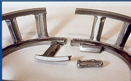
■ Phenomenon: Retainer Broken ● Cause: Excessive Vibration or Impact during Operation
